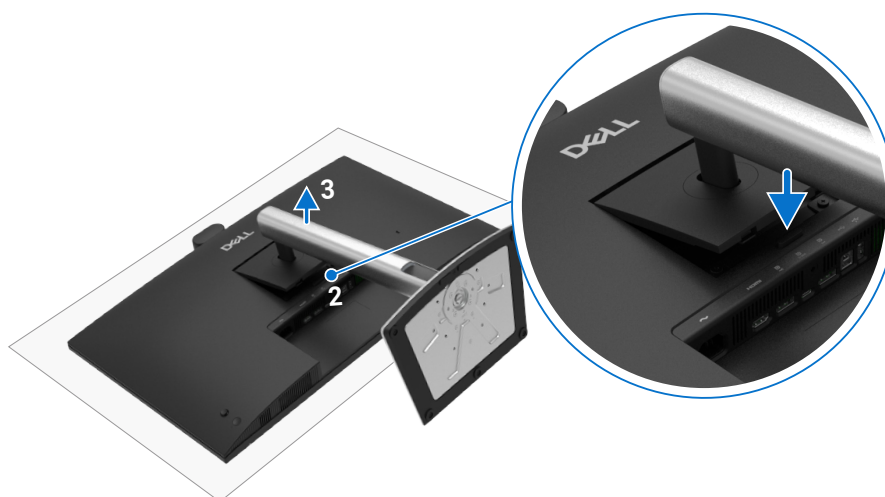
Figure 60. Removing the monitor stand
