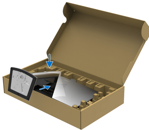
Figure 22. Insert the tabs on the stand riser into the slots
