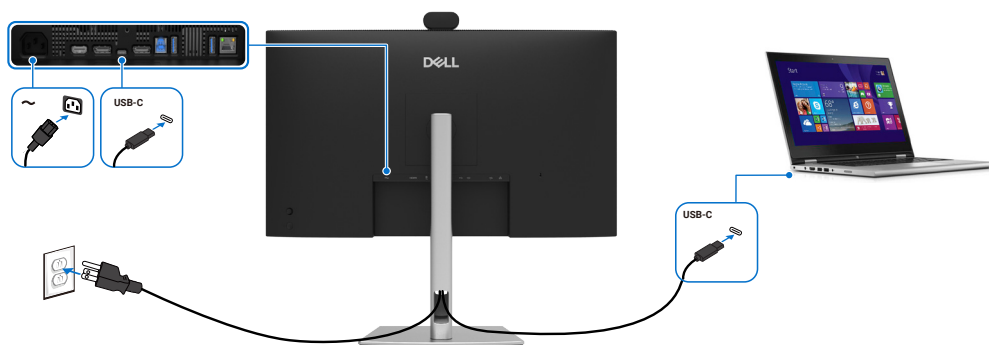
Figure 39. Connecting the USB-C cable
